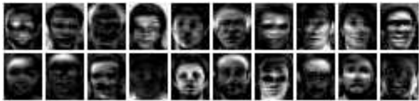
Fig. 1. Exemplary 20 basis images learned by NMF, from ORL face images, are shown. These basis images are closer to holistic representation, rather than parts-based representation, which is not a desirable characteristics of NMF.
