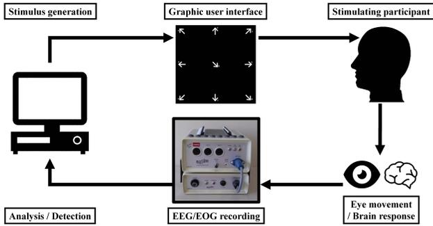
Fig. 1. Overview of the EEG-EOG hybrid BCI system
