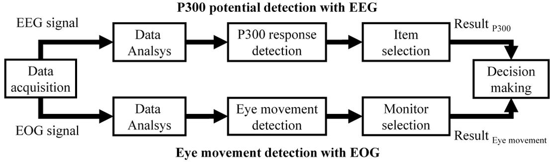
Fig. 4. In this hybrid system, EEG and EOG systems were separately analyzed. P300, which was detected from EEG signals, was used to find focused item and eye movement, which was found with EOG signals, was exploited to identify aimed monitor.
